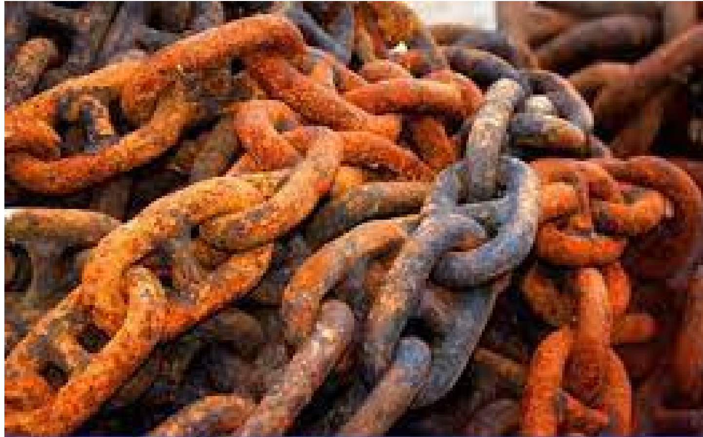
Rusting in iron chains
